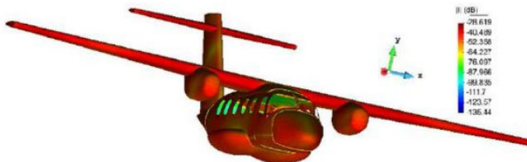
Figure 1: Surface currents on an aircraft model from a boundary element simulation with around 2 million unknowns.
